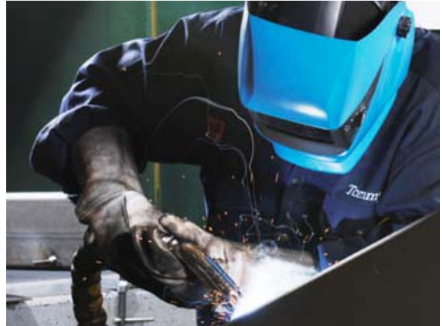
Welding torch with integrated fume extraction
