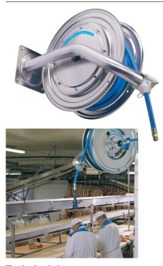
This hose reel, made entirely of stainless steel, is designed specifically or the food processing industry. It is very easy to clean thanks to rounded edges and features an easy to dismantle hose outlet, an externally mounted swivel, and a minimum number of material joints.
