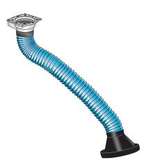
The Nederman Telescopic arm is specially designed for working environments with fumes, vapours or non explosive dust, where the space is limited. Typical workplaces can be welding schools or for production in small welding booths. The applications can be welding, grinding, or other industrial processes where a small, easily positioned arm is required. The reach of the arm is between 0.9 and 1.6 m (3 and 5 ft.).
