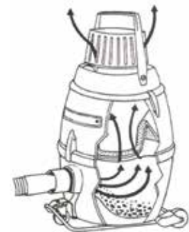
Stages of filtration
